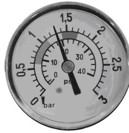
**1,3 kg/cm<sup>2</sup> - 18,5 PSI:** This pressure indicates that it is necessary to **"BACKWASH"**
