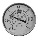
**0.8 kg/cm² - 11.4 PSI:** Normal pressure at the beginning of a filtering cycle.
