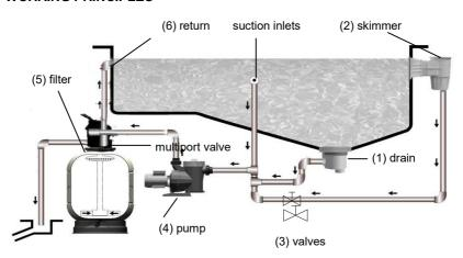
Suction is taken from the main drains (1) on the bottom of the pool and the skimmers (2) at the pool surface and fed via separate pipe work with their corresponding valves (3), through the pump (4) to the sand filter (5).
